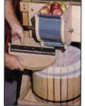
3. When tub is full, fold ends of pressing bag over pulp, add wooden pressing plate and lower the pressing screw.
