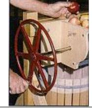
2. Turn flywheel as fast as you can. Pulp falls into tub.
