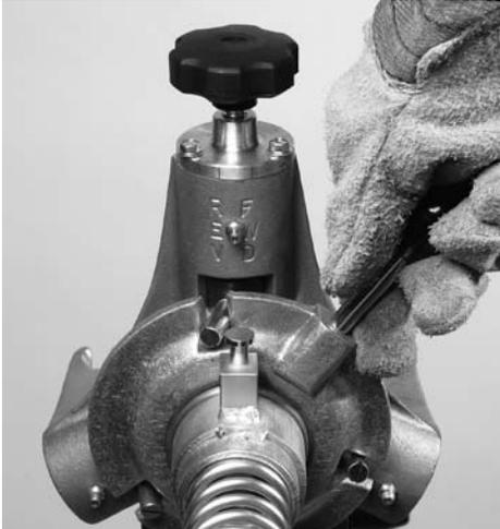
9. After tool has been removed from obstruction, move control lever back to the **FORWARD** position and continue to work through obstruction.
