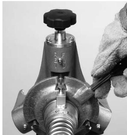
**DANGER: NEVER** force the cable or tool into the obstruction. Choose the proper feeding speed in order to give a smooth cutting action.
