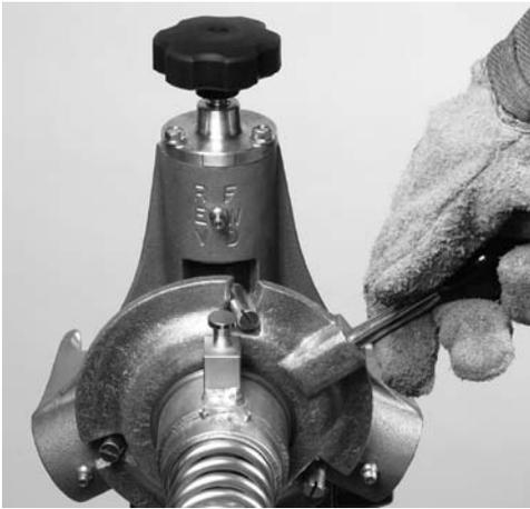
**NOTE:** The speed at which the cable is fed initially can be controlled by moving the control lever toward **FORWARD** to increase speed and moving back toward **NEUTRAL** to slow speed.
