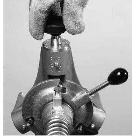
7. Continue to automatically feed cable until obstruction is met. When cable begins to drag or rotation becomes difficult, move the lever to the **NEUTRAL** position and allow tool to cut away at the obstruction. (See Figure #4 for **NEUTRAL** feeder position)
