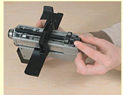
Micrometric measure for easy adjustment of strip width.
