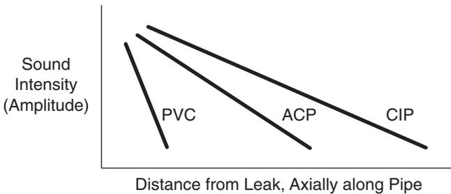
**Figure 4-5 Sound Transmission vs. Distance from Leak**
