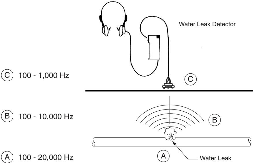
**Figure 4-3 Absorption of Sound Frequencies by Soil**
