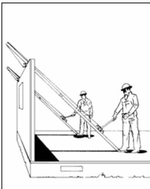
When the wall reaches the upright position, it is stopped and held firmly by the preset wall stops, which are adjustable.
