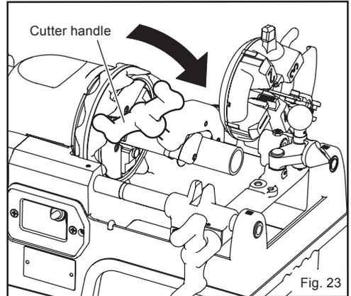
When cutting a stainless steel pipe, use a **stainless steel pipe cutter wheel (product code: 135071)**.
