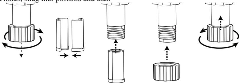
Fig. 8 - Hand tighten ONLY. No Tools.
