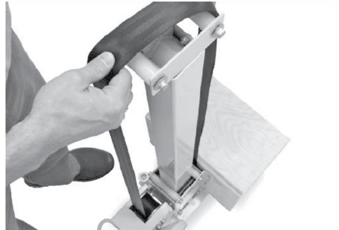
5. Position the strap over the top rollers, making sure that it is aligned straight with no twists.
