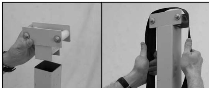
7. Insert the top roller assembly then position the strap over the top rollers, raising the Collar up the Boom.
