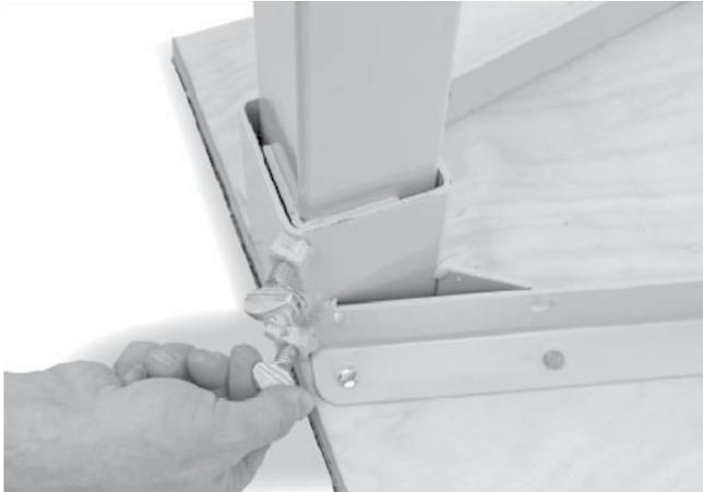
2. Tighten the thumb screws on the Counter Base to hold the Boom firmly in place.
