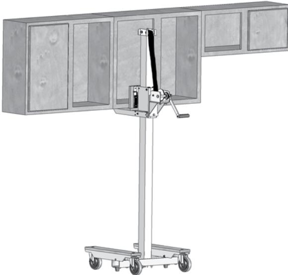
2. -Operate the winch to raise cabinets into place.
