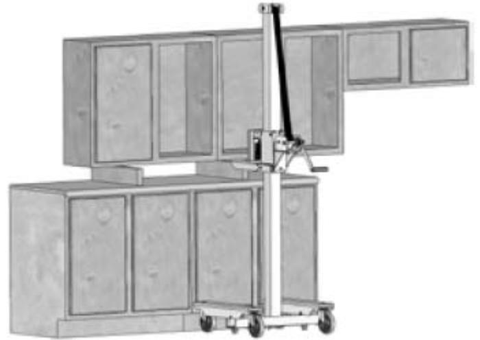
1. Start by using the Dolly Base Assembly to raise the upper cabinets to blocks (approx. 9" high, blocks not included) on the base counters.
