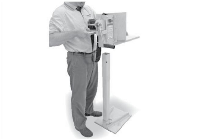
3. Let out a 2' loop of strap on the Collar Assembly and slide the Collar Assembly over the Boom Tube. **MAKE SURE** the seat of the Collar Assembly is oriented on the same side as the Counter Base as shown.
