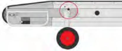
3. Fit hopper to base of machine. Align the slots both sides so they line up with the dome head pins. Pins are shown in **red**. (Fig. 3.) Push hopper toward top of machine until the domed pin stops at the base of the slot. Then push down to lock hopper in place. (Fig. 4.)
