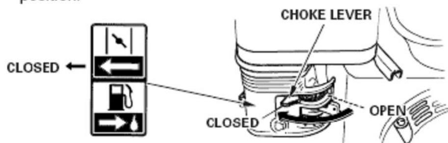
To restart a warm engine, leave the choke lever in the OPEN position.
