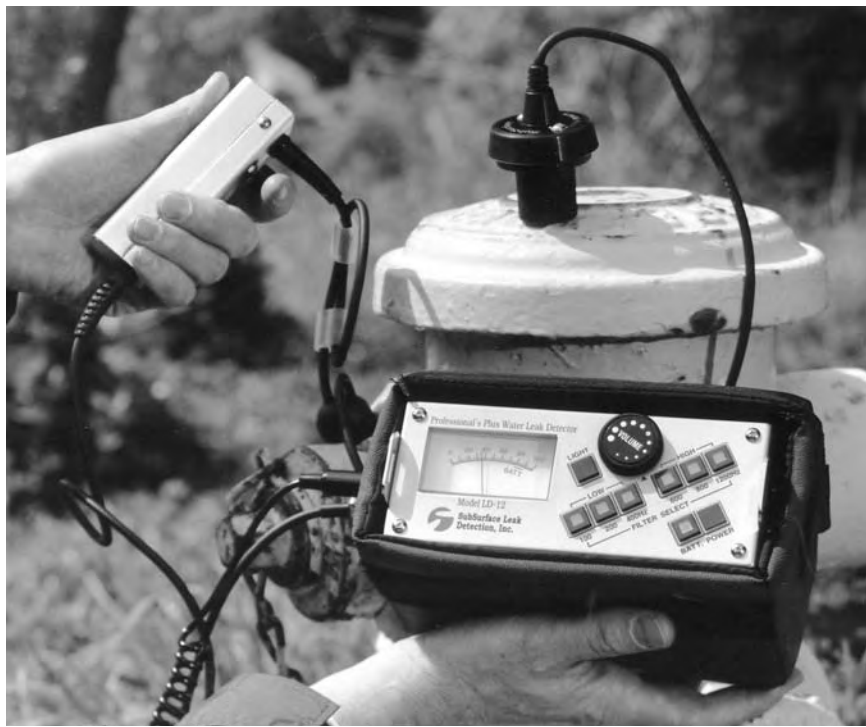
Figure 4-6 Leak Survey at a Hydrant
